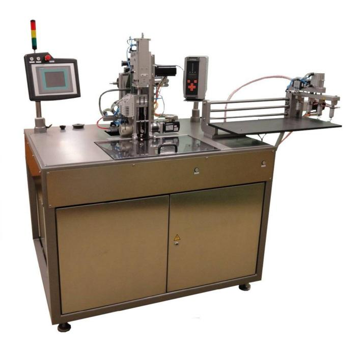
US-Sealing machine for RFID-antennas sealed off the roll to sheet mounted on the right 4-fold taker station 35 cycles per minute
