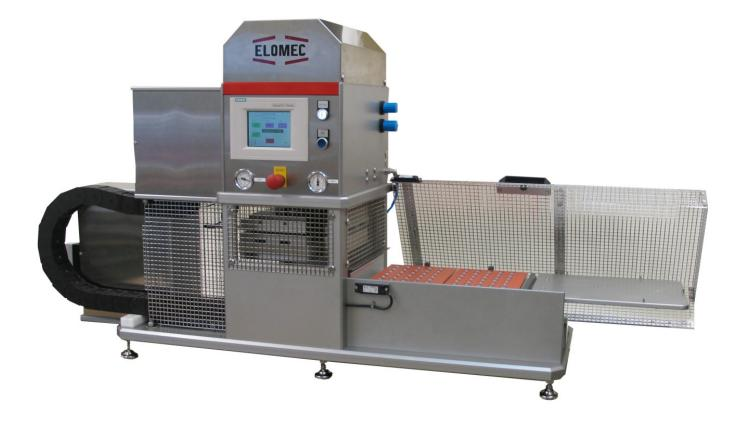
Sealing machine with two sealing units for medication blister
