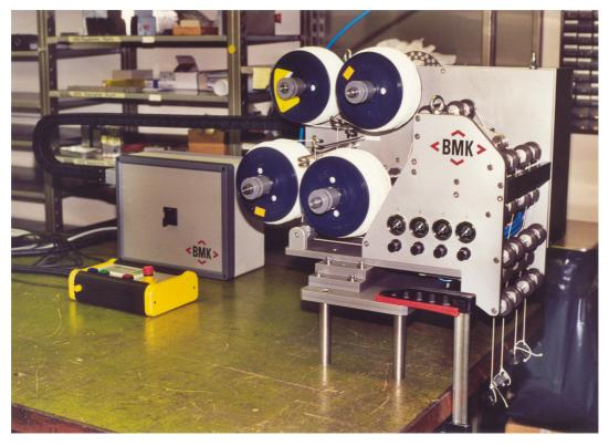
Rolling unit for 4-fold cord in spraying machine
